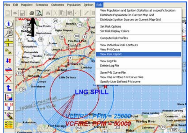
Risk Contours, dispersion, radiation and explosive effects can be overlaid on maps
